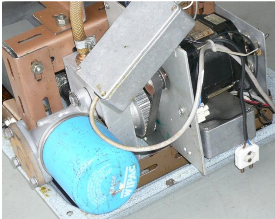
Belt-driven oil pump with mounting block and motor
