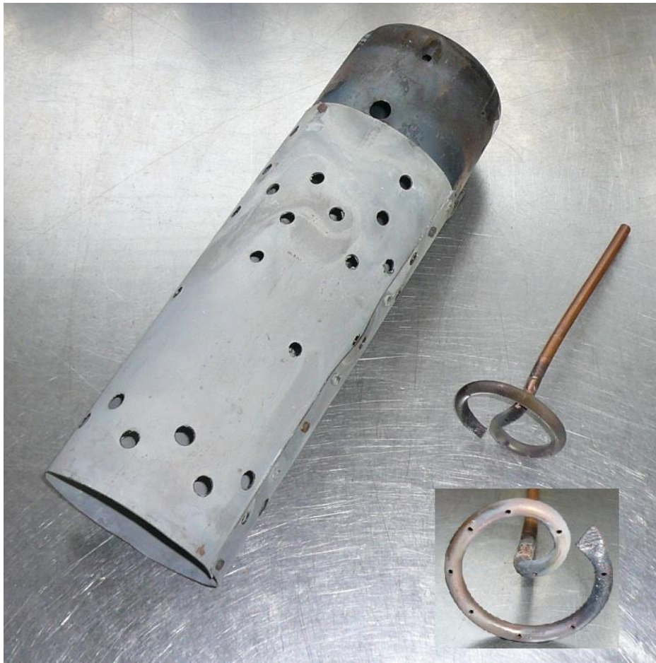
Combustion chamber liner/flame tube with burner ring (inset)
