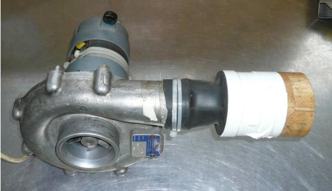
Motor driven blower unit used for starting
