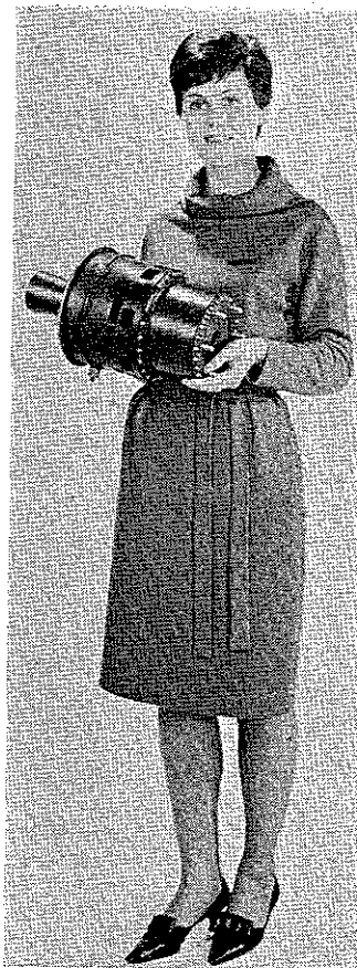
Fig. 3 Showing comparative size of gas turbine type GT-15. Turbine section with exhaust pipe on the left, gearbox on the right. Dry weight of engine, fully equipped, 22 lb. Rated power 15 hp at sea level, 25 C ambient temperature
